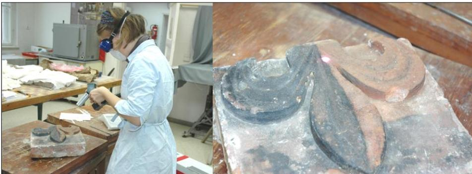
Figure (10) Shows cleaning of a ceramic architectural detail by laser ablation using a laser developed in the Military Academy of Technology in Warsaw (WAT) by Prof. Jan Marczak (photo by the author)
